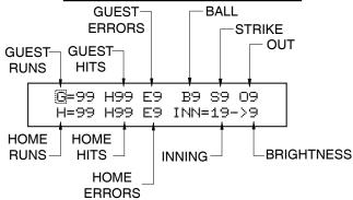
AT BAT INDICATOR: Press and Release A.B.I. button once to toggle the indicator back and forth between home and guest. Cursor moves back and forth in the LCD screen to highlight G=99 or H=99. To set the number display, press and release the AT BAT button once to increment by one. Or press and release the AT BAT button once and then select a number from 0-19 on the keypad.
